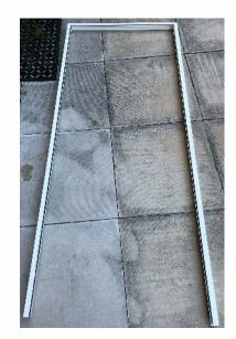
2. Position this frame onto the door frame where you want it to be fixed and make sure it is straight using a spirit level and then mark the upright positions using a pencil
