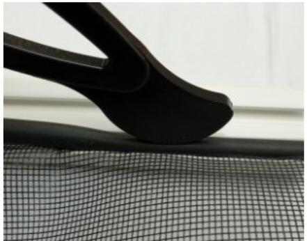
3. Lay the assembled frame on a flat surface with the inner groove facing you. Place the mesh over the panel and start to push the rubber gasket into the groove using the tool supplied. Trim off any excess mesh with a sharp Stanley knife.
