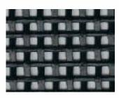
Construction - fibreglass / PVC ultrasonically welded Density - warp 16 / weft 14 , approx 50% openness factor Weight - grams per sq mtr / ca. 20g +/- 10% Thickness - ca 0.31mm +/- 0.05%
