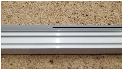
Drill hole at rear
